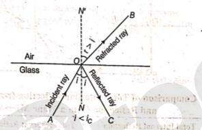
Case 2 When the angle of incidence is equal to critical angle,  $(i = i_C)$
