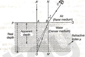
Refractive index  $\mu = \frac{OA}{IA} = \frac{\text{Real depth}}{\text{Apparent depth}}$
