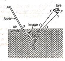
The rays of light coming from tip O of the stick when passing from water to air, bend away from the normal and appear to be coming from a point L, which is the virtual image of the point O. It is true for every point of the stick inside the water.
